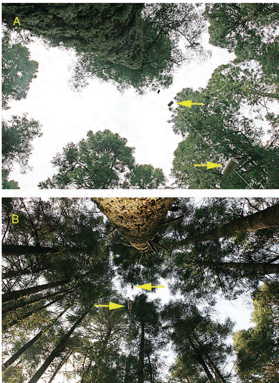
FIG. 3. The experimental trees. (A) view of the vertical transect at Tree 1; (B) same, Tree 2. Four of the eight cylinders in which the Thermochrons were mounted are visible in A, while two are visible in B; two cylinders in each photo are marked by arrows. The canopy above Tree 1 is 34% open to the sky, and Tree 2 is 13% open. (Photos, L. P. Brower, from the same facing angles as the transects.)
