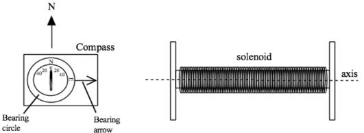
b) Devise an experiment to determine the relationship between the solenoid's B-field and the current through the coil. Write the procedure in your notebook. Be sure to record and use uncertainties. Also take advantage of reversing the current to further reduce alignment error. Between measurements turn off the power supply and check that the apparatus is aligned properly and that the solenoid is not too hot.
