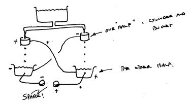
How does this happen? Let's assume an initial asymmetry of charge between the two copper cylinder-bucket halves. (It doesn't matter how small this is.) The cylinders have electric fields like this
