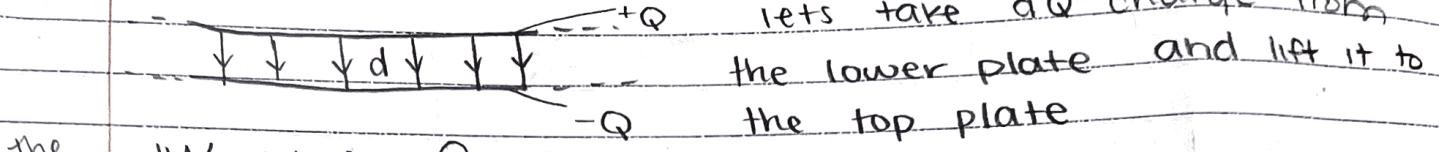
$$\text{the work: } dW = VdQ = \frac{Q}{C} dQ$$
