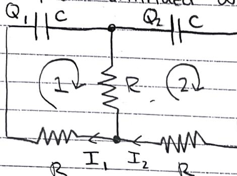
$$\text{nodes: } I_1 = I_2 + I_3 \Rightarrow I_3 = I_1 - I_2$$
