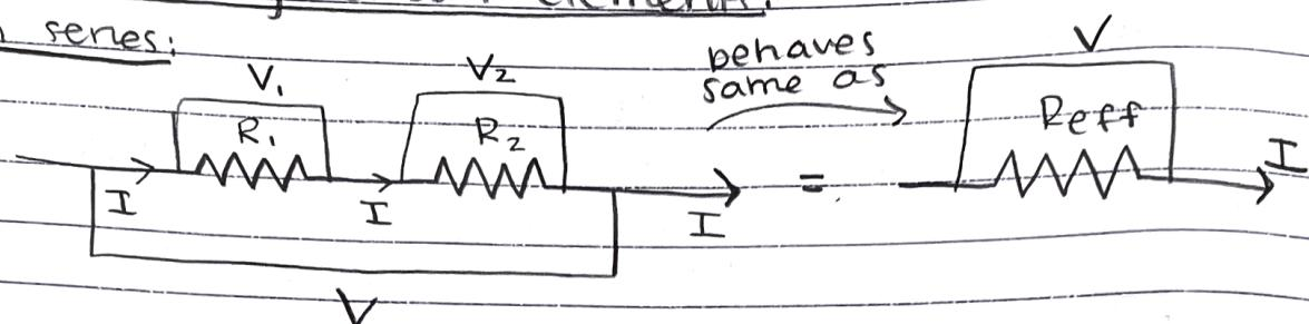
$$V = IR_{\text{eff}} = IR_1 + IR_2 \quad ] \quad \text{currents are constant;}$$
